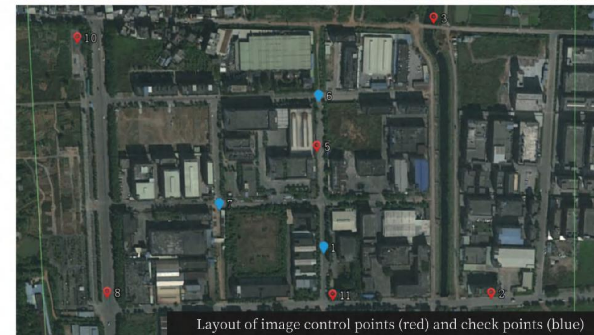
Layout of image control points (red) and check points (blue)
